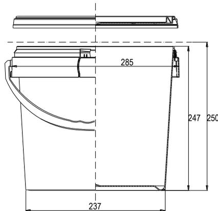
Measurements in millimetres
